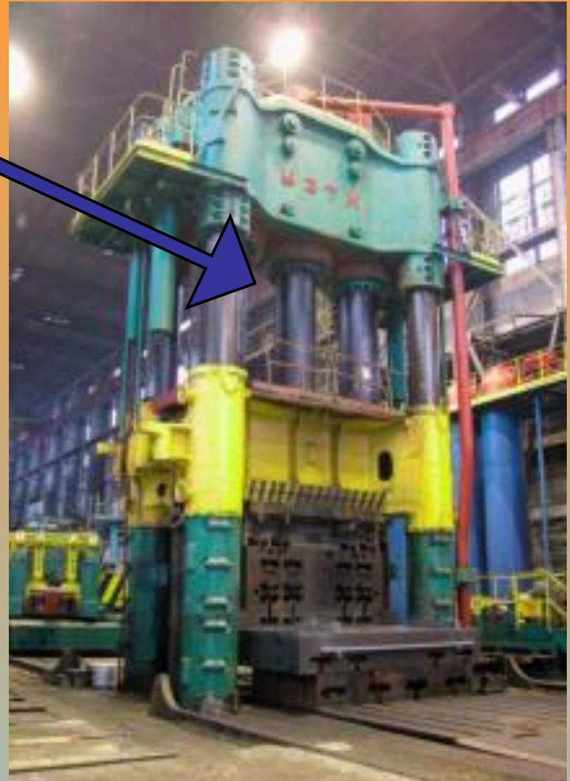
***VEE-PACKING LIFE IS CRITICAL IN OPEN DYE FORGING PRESSES.***
